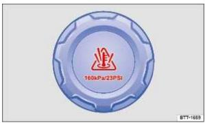
Fig. 173 In the engine compartment: coolant expansion tank cap (illustration).
