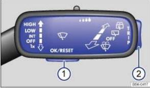
Fig. 19 On the right of the steering column: buttons on the wiper lever (illustration).
