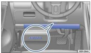
Fig. 41 On the driver side: location of the knee airbag.
