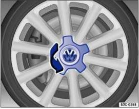
Fig. 182 Removing the centre wheel trims by turning.
