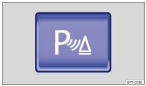
Fig. 111 In the centre console: button for switching Park Distance Control on and off (depending on equipment).
