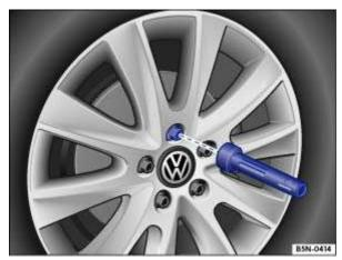
Fig. 189 Changing the wheel: removing the wheel bolts with the screwdriver handle.
