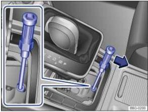
Fig. 96 Unlocking the selector lever lock manually.
