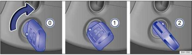
Fig. 90 To the right of the steering wheel: positions of the vehicle key in the ignition lock.
