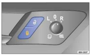
Fig. 55 In the driver door: central locking button.
