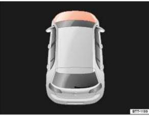
Fig. 170 On the instrument cluster display: the bonnet is open or has not been closed properly.
