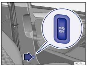
Fig. 59 Next to the driver seat: button for switching off the interior monitoring system and anti-tow alarm (depending on vehicle equipment).
