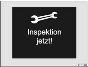
Fig. 18 In the instrument cluster display: example of a display in the instrument cluster when a service is due (illustration).
