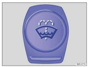
Fig. 171 In the engine compartment: cap of washer fluid reservoir.
