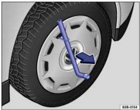
Fig. 183 Removing the wheel covers.
