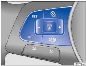
Fig. 105 Left-hand side of the multifunction steering wheel: buttons for operating ACC.
