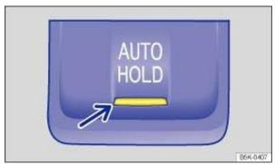
Fig. 110 In the centre console: button for the Auto Hold function.
