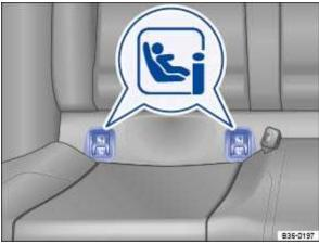
Fig. 46 On vehicle seat: markings identifying the ISOFIX anchor points for child seats (illustration).
