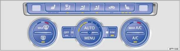
Fig. 86 In the upper part of the centre console: Climatronic air conditioning block.
