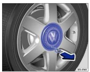
Fig. 181 Removing the centre wheel trims by pulling.
