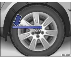
Fig. 185 Changing a wheel: loosening the wheel bolts.
