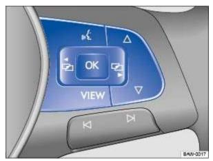
Fig. 20 Right-hand side of the multifunction steering wheel: controls for using the menus and information displays in the instrument cluster.
