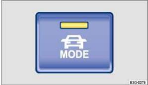
Fig. 97 In the lower part of the centre console: button for selecting driving profile
