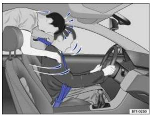
Fig. 27 The unbelted rear passenger is thrown forwards, hitting the belted driver.
