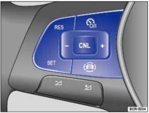
Fig. 99 Left-hand side of the multifunction steering wheel: buttons for operating the CCS.
