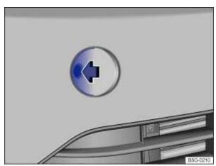
Fig. 166 In the right-hand side of the front bumper: removing the cover.
