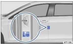
Fig. 178 On the driver door pillar: tyre pressure sticker (alternatively on the inside of the charging socket flap).
