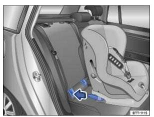
Fig. 47 Fitting a typical ISOFIX child seat with the attachment arms.
