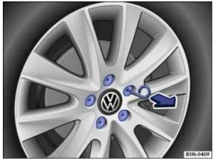
Fig. 184 Removing the wheel bolt caps.
