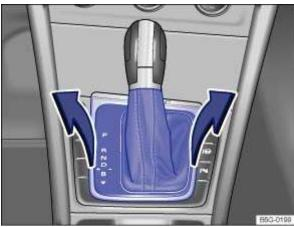
Fig. 95 Removing the cover of the gearshift gate.
