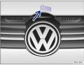
Fig. 169 Above the radiator grille: bonnet opening lever.
