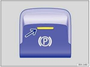
Fig. 109 In centre console: button for the electronic parking brake.
