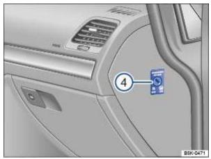
Fig. 11 With open front passenger door (left-hand drive vehicles): key-operated switch in the dash panel (mirrored for right-hand drive vehicles).
