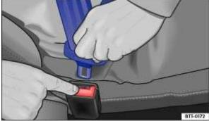
Fig. 30 Removing the latch plate from the buckle.
