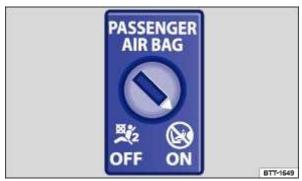
Fig. 37 In the dash panel on the front passenger side: key switch for disabling and enabling the front airbag on the front passenger side
