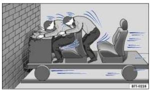
Fig. 25 Unbelted occupants in a vehicle striking a brick wall.
