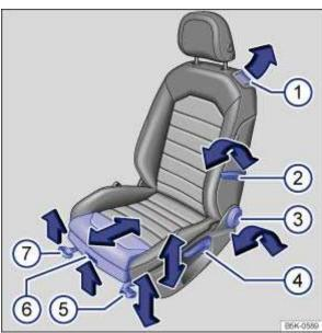
Fig. 65 On the left front seat: controls.
