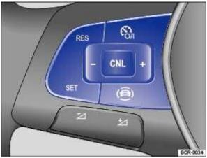
Fig. 101 Left-hand side of the multifunction steering wheel: buttons for operating the speed limiter.
